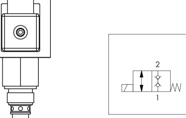
OPERATING PRESSURE- PORT 1-210 BAR, PORT 2-315 BAR FLOW- 30 L/min(8GPM)
